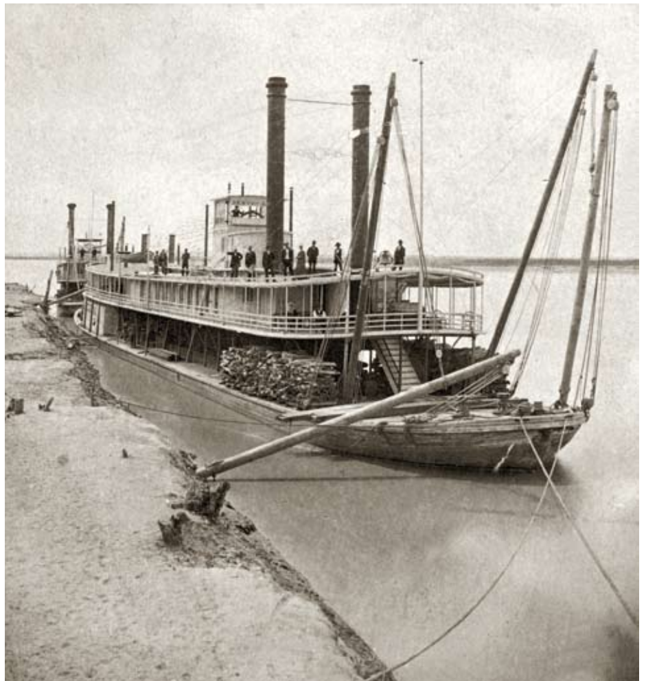
FIGURE 12.6: Steamboats required enormous supplies of firewood to feed their engines. Steamboat companies hired woodcutters (called "woodhawks") to cut and stack firewood along the Missouri River so the steamboats could reload as they progressed upriver.
