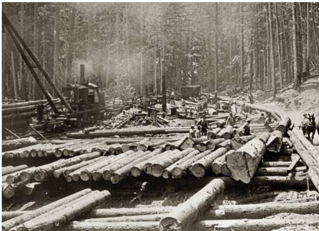
FIGURE 12.11: One of the easiest ways to move logs overland was along a greased chute. Here lumberjacks roll logs off the chute (far right) for loading onto a railroad donkey engine, which transported logs to the mill.
