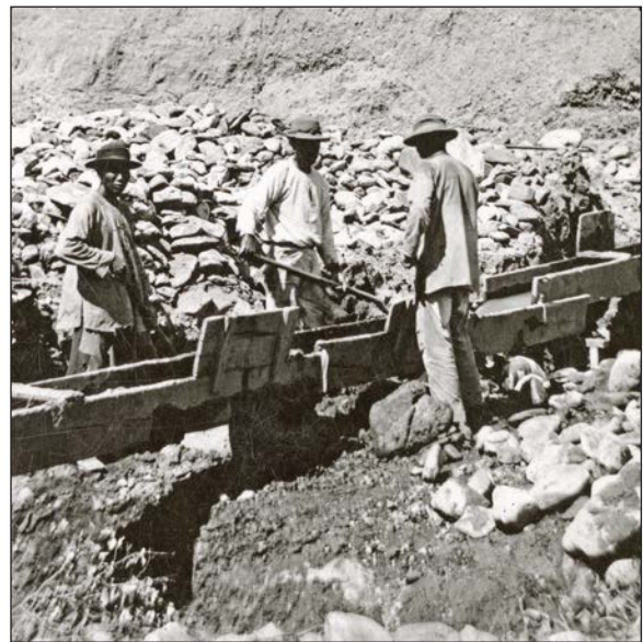
Working together in 1871, these Chinese miners used a sluice box to help them separate gold from the dirt and rocks.
