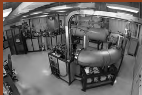
Radiocarbon dating is now most commonly done with an accelerator mass spectrometer. U.S. Dept. of Energy
