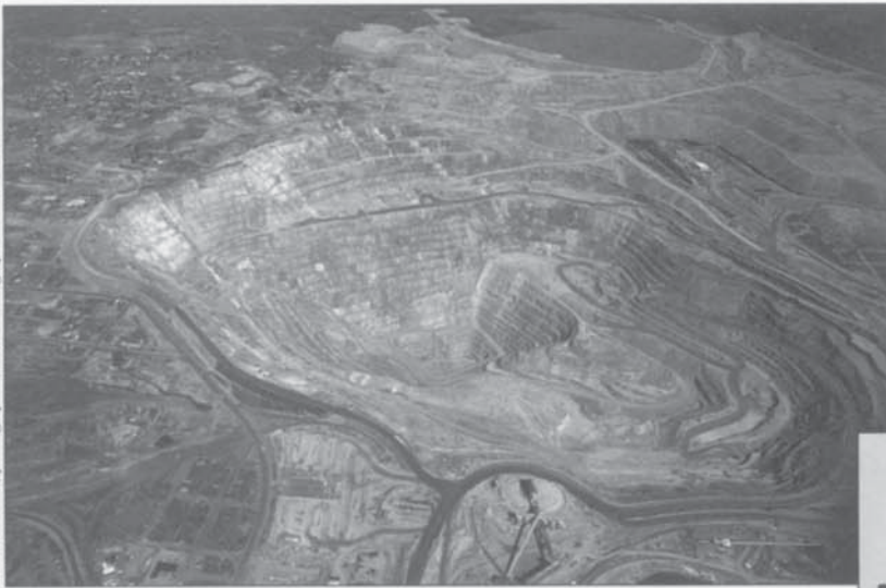
Aerial view (above) shows the Anaconda Company's Berkeley Pit in operation in the 1970s. Today, with underground pumps shut down, the pit is filling with acid water at the rate of two and a half million gallons a day.
